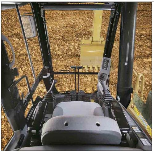
**Cab Design.** The workstation is spacious, quiet and comfortable, assuring high productivity during a long work day. The air conditioner and attachment switches are conveniently located on the right-hand wall, and the key switch and throttle dial are on the right-hand console. The monitor is easy to see and maximizes visibility.
